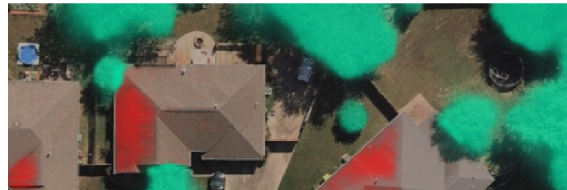
Nearmap AI automatic feature detection tool shows areas of medium to high vegetation (green) and tree overhang (red).
